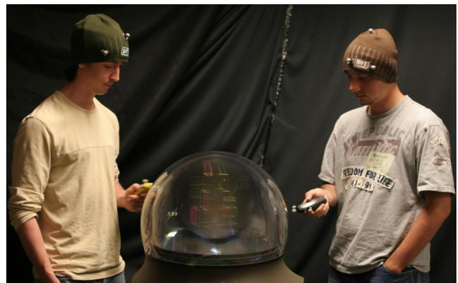
**Figure 1. The prototype for our explorations allowed users to collaboratively interact with the volumetric display. Users' viewing positions and input devices were tracked in 3D.**
