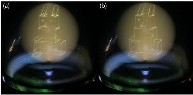
**Figure 9. a) Typically volumetric displays are incapable of hidden surface removal. b) The same scene displayed using our hidden surface removal algorithm, which is updated in real-time based on the user's viewpoint. For illustration in this figure, the algorithm is based on the location of the camera.**
