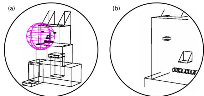
**Figure 4. Zoom-In Tool. a) The user controls the position and radius of a spherical 3D cursor. b) Clicking the left button zooms in to the area represented by the sphere. Circles represent the display volume.**
