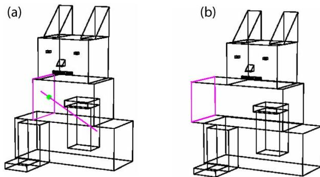
Figure 7. The depth ray (a) can select and drag faces (b).
