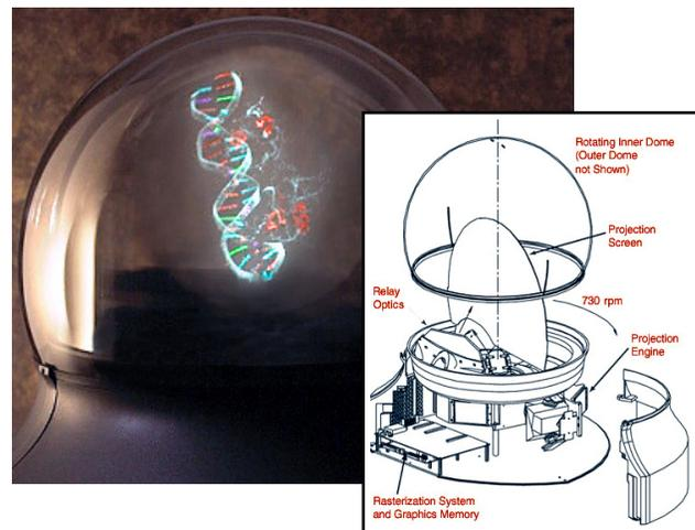
Figure 2. Actuality System’s volumetric display.
