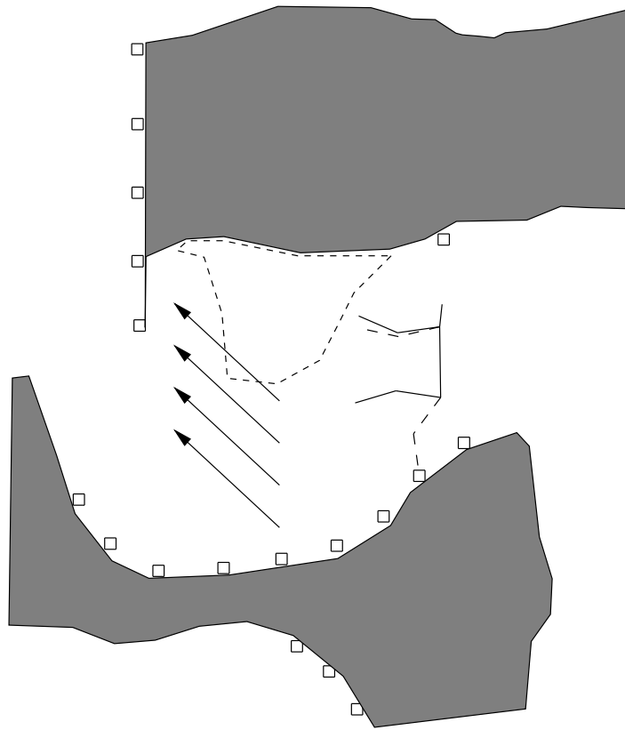
Figure 5.13: A weakness of the planner due to the use of simplified inverse kinematics; the arrows show the gradient of the distance map
