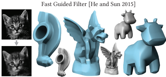
Fig. 14. We generalize the fast guided filter to 3D and achieve edge-preserving smoothing effect.
