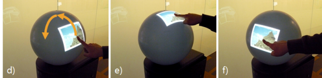
Figure 9: Comparison of orientation difficulties when dragging an object along a similar path shown in (a) and (d): (a–c) default unassisted behavior results in a difficult object orientation visible in (c); (d–f) Auto-rotation behavior eliminates such problems by continuously orienting objects with respect to the top.
