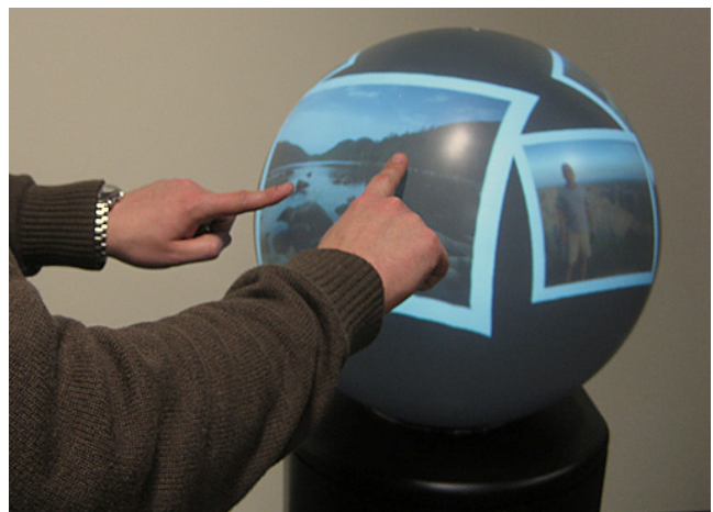
Figure 1: Scaling a picture on Sphere, a multi-user, multi-touch spherical display prototype built on top of a Magic Planet display.
