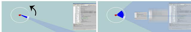
Figure 5. Close-up of scaling vacuum. As the arc is increased to include the window item (left image), a copy of the item is scaled down and brought to the tool's centre (right image). Motion blur in right image illustrates the animated transition that occurs during the item's movement.
